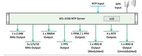
The VCL-2156 is equipped with a highly accurate, low-noise OCXO to provide a high stability, ITU-T G.812, Type II, III compliant holdover clock with better than 12µs accuracy over a 24 hour (5 milliseconds per year) period in the event of unavailability of the GPS / GNSS signal, or GPS / GNSS antenna failure, or a temporary loss of reception in a totally isolated network without any external
